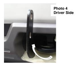
**Step-3** Hook the slot in the bracket over the shank of the front tow hook bolt, reinstall the front bolt nut and rear tow hook bolt to secure the bracket to the side of the frame, (Photo 5). Leave the nut and bolts loose for final adjustment.
