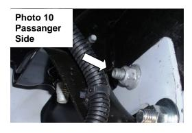
**Step-6** Attach the passenger side auxiliary bracket to the side of the frame using the tow hook rear bolt and to the passenger side main bracket using (1)  $\frac{1}{2}$ " x 1  $\frac{1}{2}$ " hex bolt, (1)  $\frac{1}{2}$ " flat washer, (1)  $\frac{1}{2}$ " lock washer and (1)  $\frac{1}{2}$ " hex nut, (Photo 11 & 12). Leave the factory and supplied nuts and bolts loose for final adjustment.
