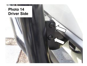
**Step-8** Align the RHINO CHARGER with the vehicle and tighten all factory and supplied nuts and bolts.
